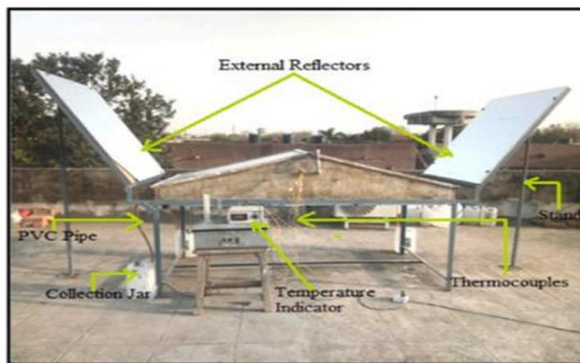
**Figure 124. Double Slope Solar Still Integrated with Externally Mounted Reflectors [51]**
