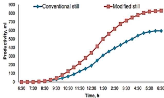
**Figure 80. Comparison of Productivity of CSS and Modified SS Proposed by Kumar et al [38]**
