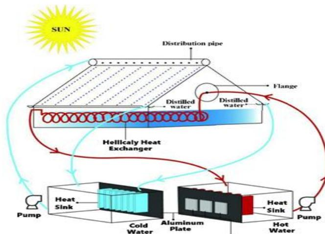
Figure 9. Thermoelectric Heater and Cooler Integrated with SS Module [36]
