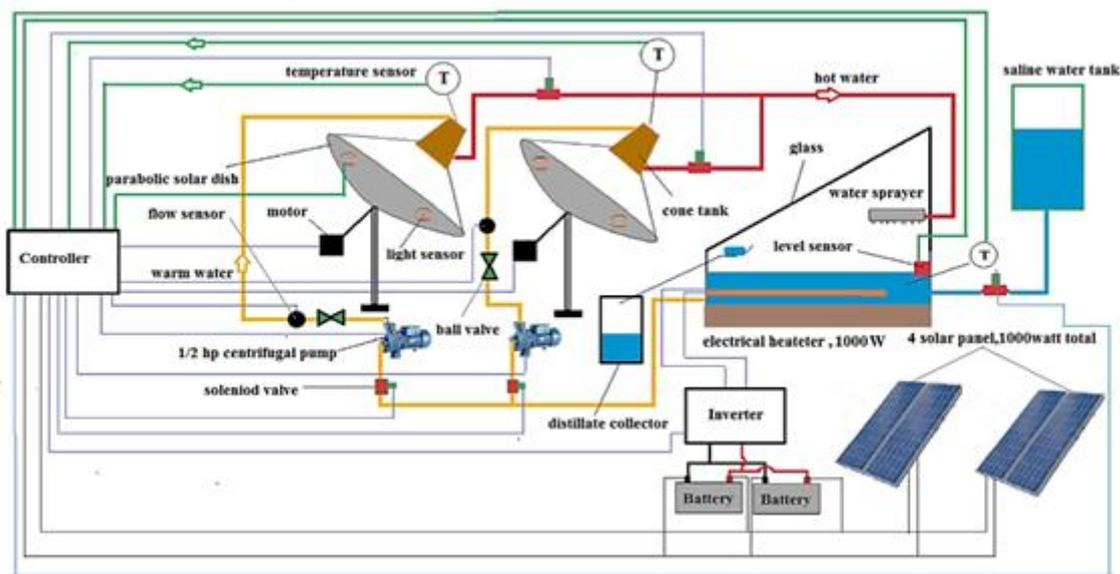
**Figure 7. Schematic Diagram for an Integration of Two Parabolic Dishes and Heat Exchanger PV - System with Single SS [29]**
