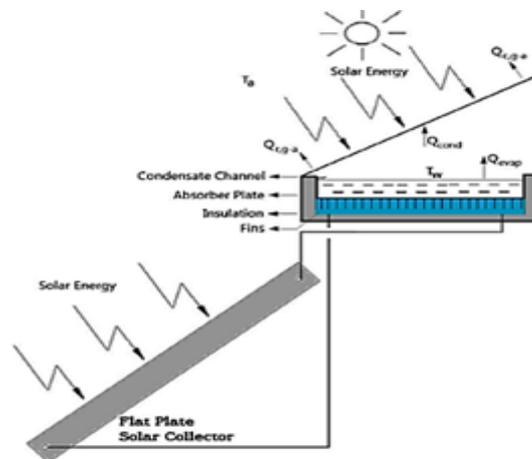
**Figure 6. Schematic Diagram of Flat Plate Solar Collector as a Preheating System Assisting Single Slope Solar Still [26]**
