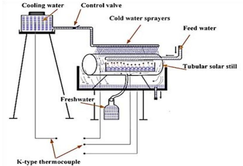
Figure 8. Schematic Diagram of Tubular Solar Still [34]
