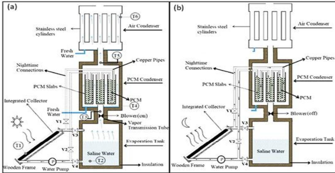
**Figure 102. The Schematic of Radiative Cooling Experimental Setup [40]**
