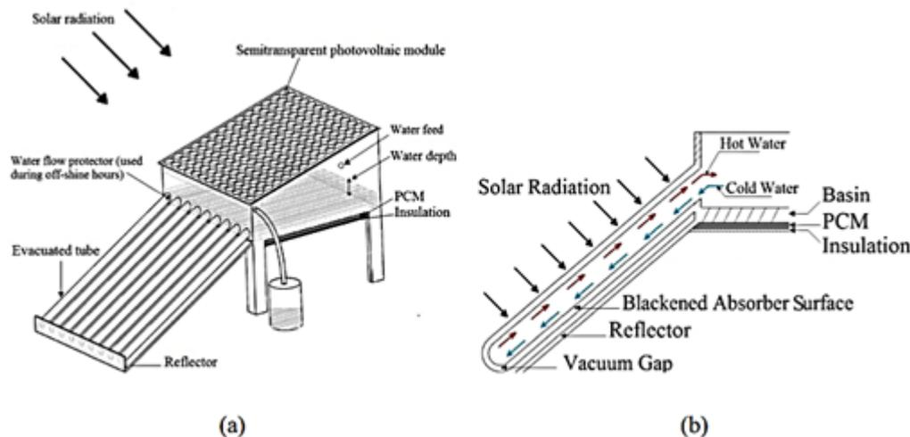
**Figure 135. a. Schematic Diagram of a Solar Still Integrated with ETC, Semitransparent PV Module and PCM, b. Schematic Diagram of Thermosiphon Process in Single Tube [55]**
