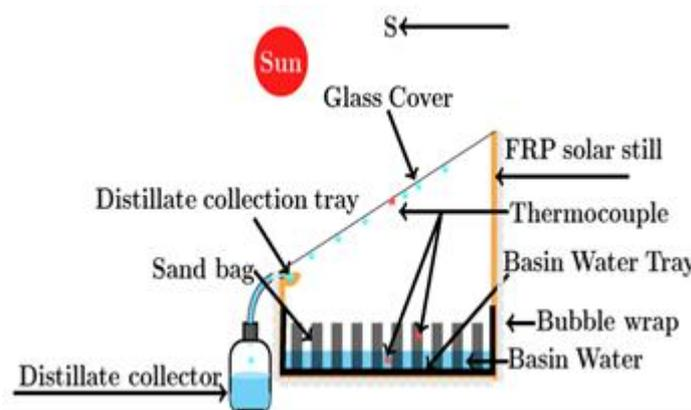
Figure 4. Schematic Representation of MSS. [22]
