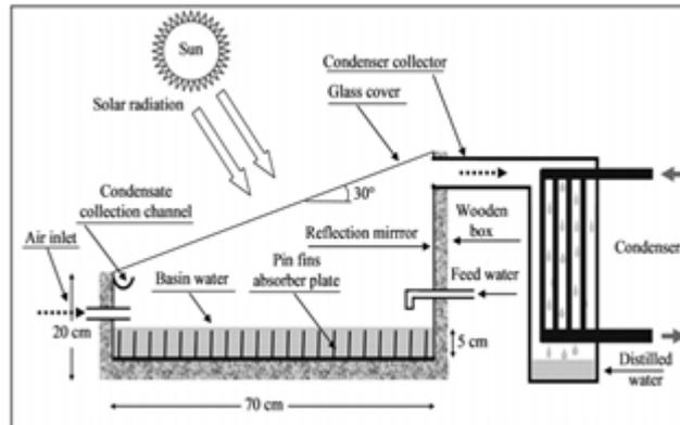
**Figure 91. The Layout of a Single Slope SS Augmented with a Pin-Fins Absorber and External Condenser [39]**
