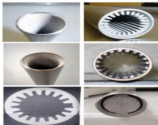
Fig. 2. Structures of wick [19].
