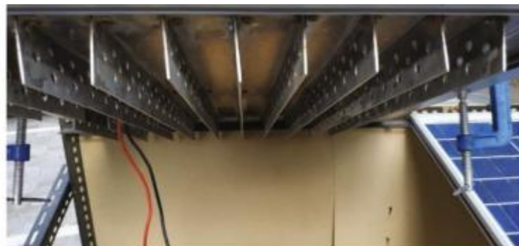
Fig. 2. Cooling system using heat sinks [37].
